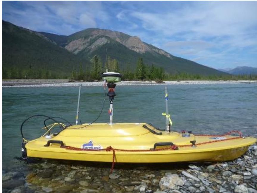
Figure 22: Z-Boat remote controlled hydrographic survey tool (image source www.survbase.com )
