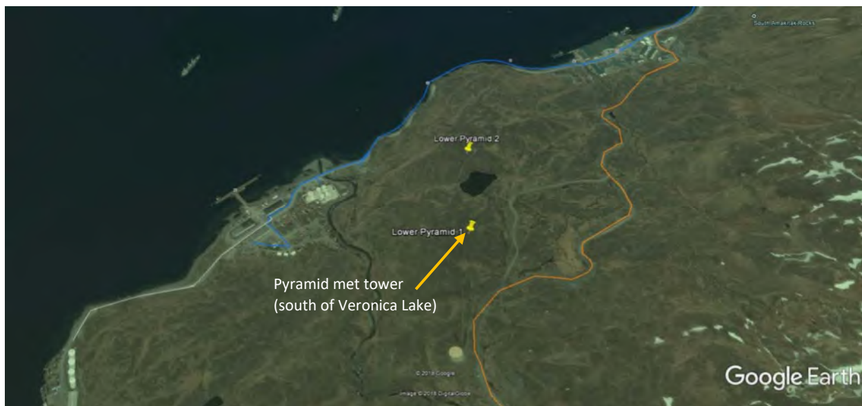
Figure 3: Pyramid met tower location (orange line shows underground power distribution routing, 3 phase to the water house/tank, continuing at single phase to Icy Creek Reservoir), view north; Google Earth image
